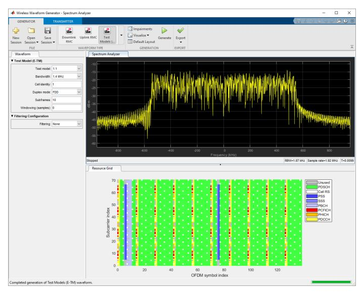
Configure the app to generate an LTE E-TM Test Model 3.1b frame with a channel bandwidth of 5 MHz. To visualize the waveform, click **Generate**.
