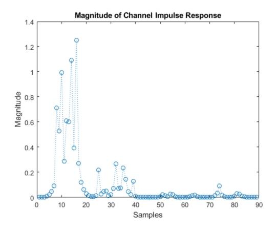
Estimate the timing offset by finding the peak of the impulse response magnitude.
